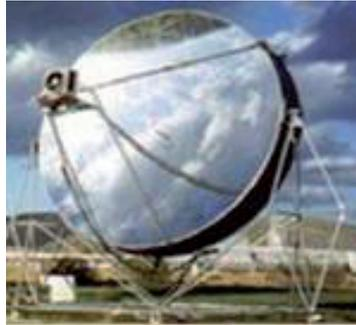
Fig. 5. Paraboloide (dish) (PSA).
